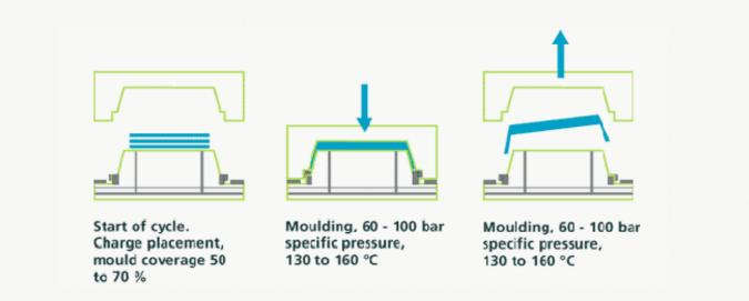
Layers of SMC are placed into the heated tool. Through closing the tool the material fills the cavity and polymerizes. After complete cure the parts are released hot.
