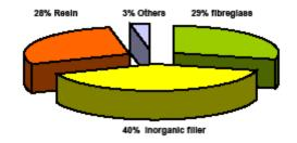
As glass fibre reinforcement in most cases cut glass rovings are used. Calcium carbonate (chalk) is the most commonly used filler. Magnesium oxide in the formulation can react with the free acid groups of the resin. This results after a few days in an enormous increase of the viscosity of the SMC formulation. A leather-like sheet is formed, which is almost non-sticky and easy to handle. In this stage the resin is still not polymerized.
