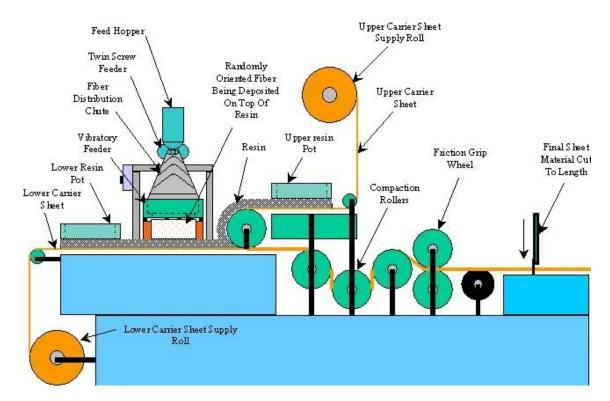
SMC is a flat sheet-like compound, produced on a continuous moving belt process. The SMC composites are made from chopped multi end rowing strand sandwiched between two layers of film, onto the resin paste (resin, shrink compensation, fillers, additives and curing agent) has already been applied. The prepreg passes through a compaction
