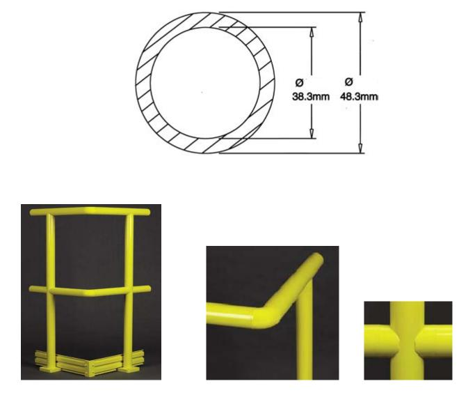
The EPP round handrail system is a round fibreglass system that is ideal for any high traffic area where handrail is needed. The round rails are easy to grip, pleasing to the eye and to the touch with 90° moulded corners which eliminate sharp edges. The handrail system meets **OSHA** strength requirements with a 2:1 factor of safety with a**1524 mm** maximum post spacing.
